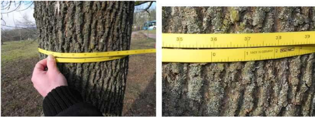
Figure 12: Measuring DBH with measuring tape for determination of diameter (here 35.9 cm).
