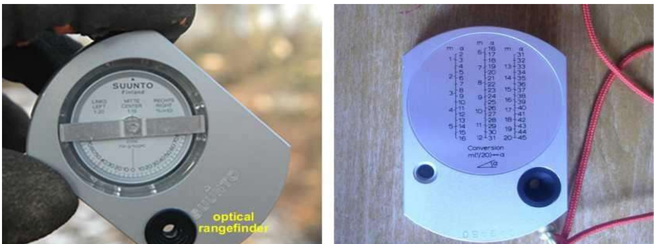
Figure 9: Hypsometer «Suunto» with optical principle for fixed distances.
